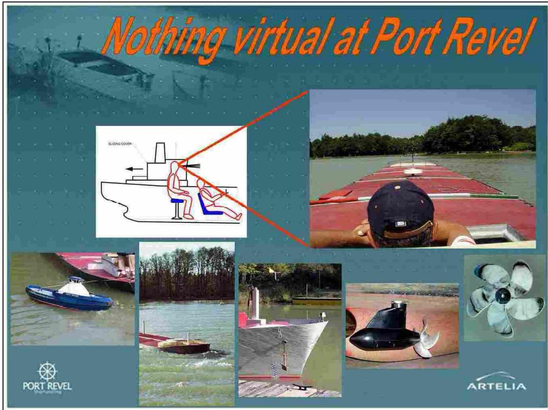
The ships are accurately constructed to conform with the principles of similitude and are fitted with indicators showing the ship's parameters. Information given by the indicators is at **full scale**.
